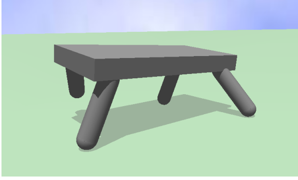
Figure 3: The quadruped robot model. The legs are attached to the body by hinge joints with axes of rotation tilted sideways, allowing the legs to make full circular rotation. Locomotion is achieved by coordinating the circular movements of the legs. This model is a simple but physically realistic platform that also allows scaling up to more complex robots by adding more legs or by increasing the legs’ degrees of freedom.
