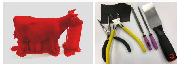
Figure 1: Left: 3D printed cow with support structure. Right: Some of the basic tools used for removing support material including pliers, a spatula, and sandpaper.
