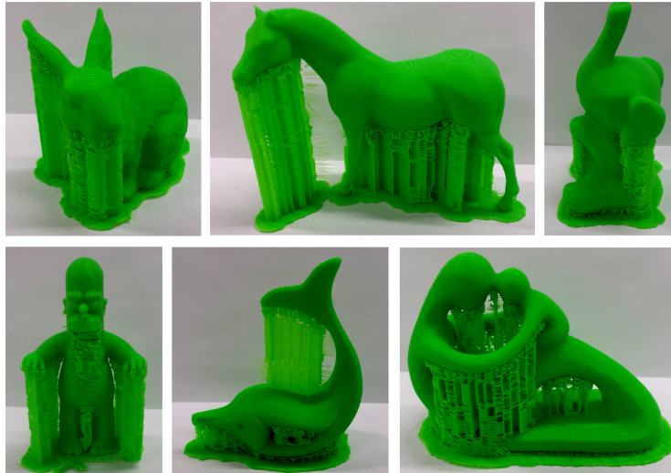
Figure 8: Original objects printed with support structures. Support structures need to be printed under overhanging areas. Supports waste material and are time-consuming to remove.
