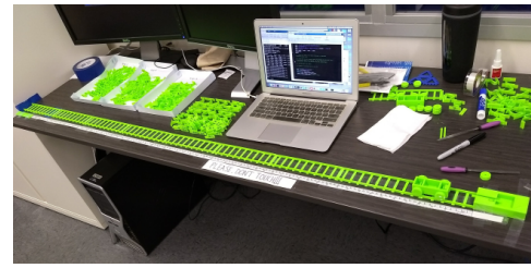
Figure 2: The green parts located along the edge of the table constitute the 3D printed car-launcher mechanism. The track has a length of 157cm and a ruler is attached next to the track for the measurements. A link to the video of the experimental setup can be found in [1].
