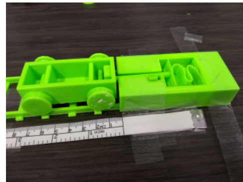
Figure 3: Closer view of the car-launcher mechanism is shown above. A test spring is loaded and ready to propel the car.
