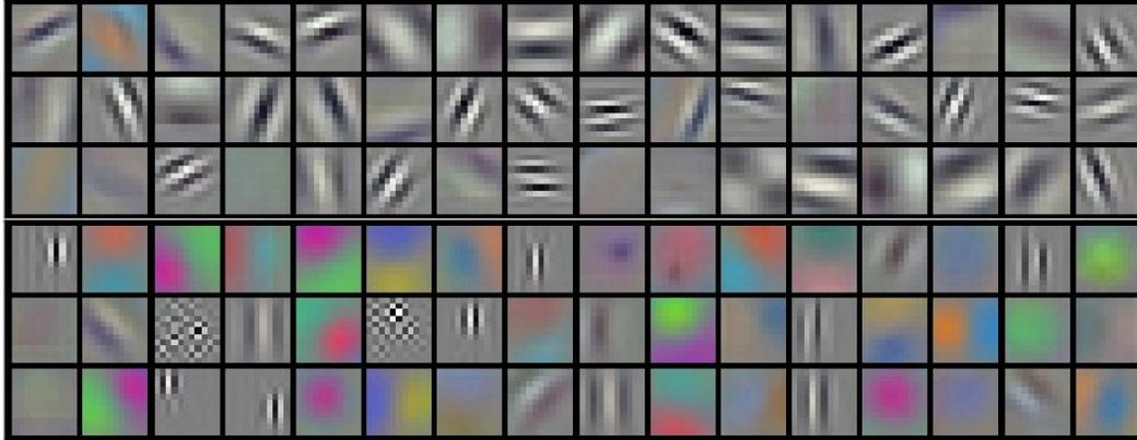
Figure 1.2: **Convolutional Filters Learned in AlexNet [9] for Image Classification.** The image shows 96 convolutional kernels of size 11x11x3 learned by the first convolutional layer in AlexNet. Deep learning is able to discover suitable features for the task of image classification. These learned features perform better than the engineered SIFT features. This example highlights the potential of learning algorithms to discover novel and effective solutions without a need for engineering.
