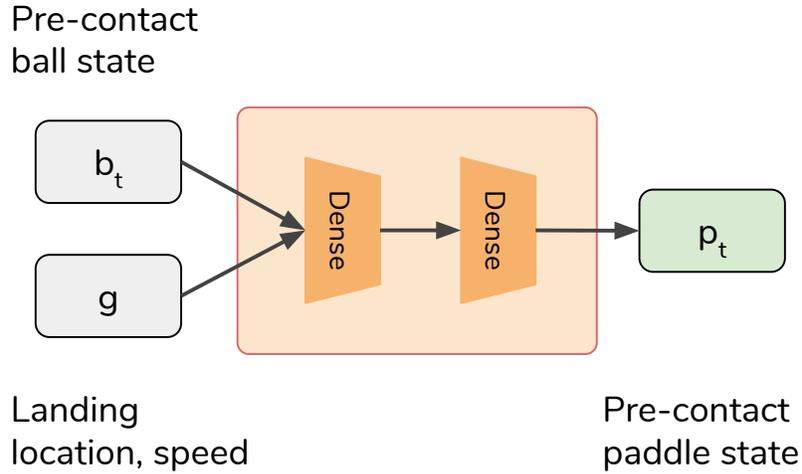
Figure 6.3: **Inverse Landing-Prediction Model.** It is a feed-forward network with two fully-connected hidden layers. Given pre-contact ball-motion state and a desired landing target, the model predicts the paddle-motion state right before contact. The predicted paddle-motion can be used as an action for the paddle-control skill.
