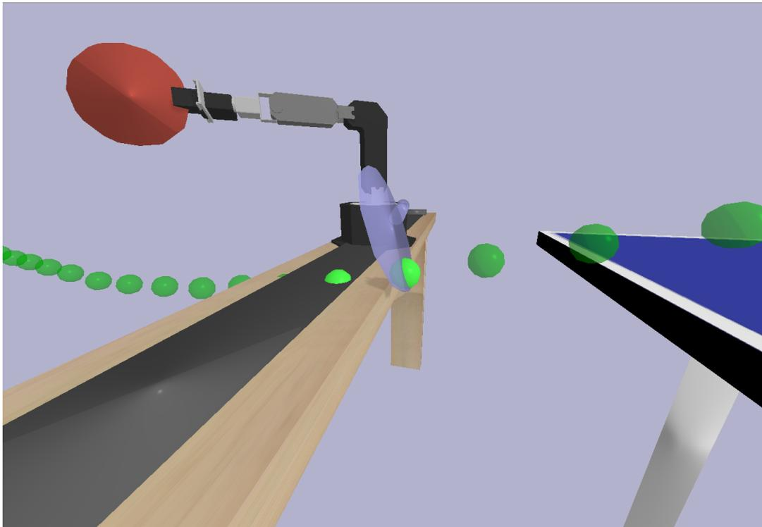
Figure 8.4: **Example Failure Case for Model-Based Land-Ball Policy.** At times, the trajectory of the launcher ball collides with the table under the robot assembly. The translucent paddle visualizes the requested paddle-motion target. Such balls are more difficult to return, as the planned paddle trajectory may collide with the table.
