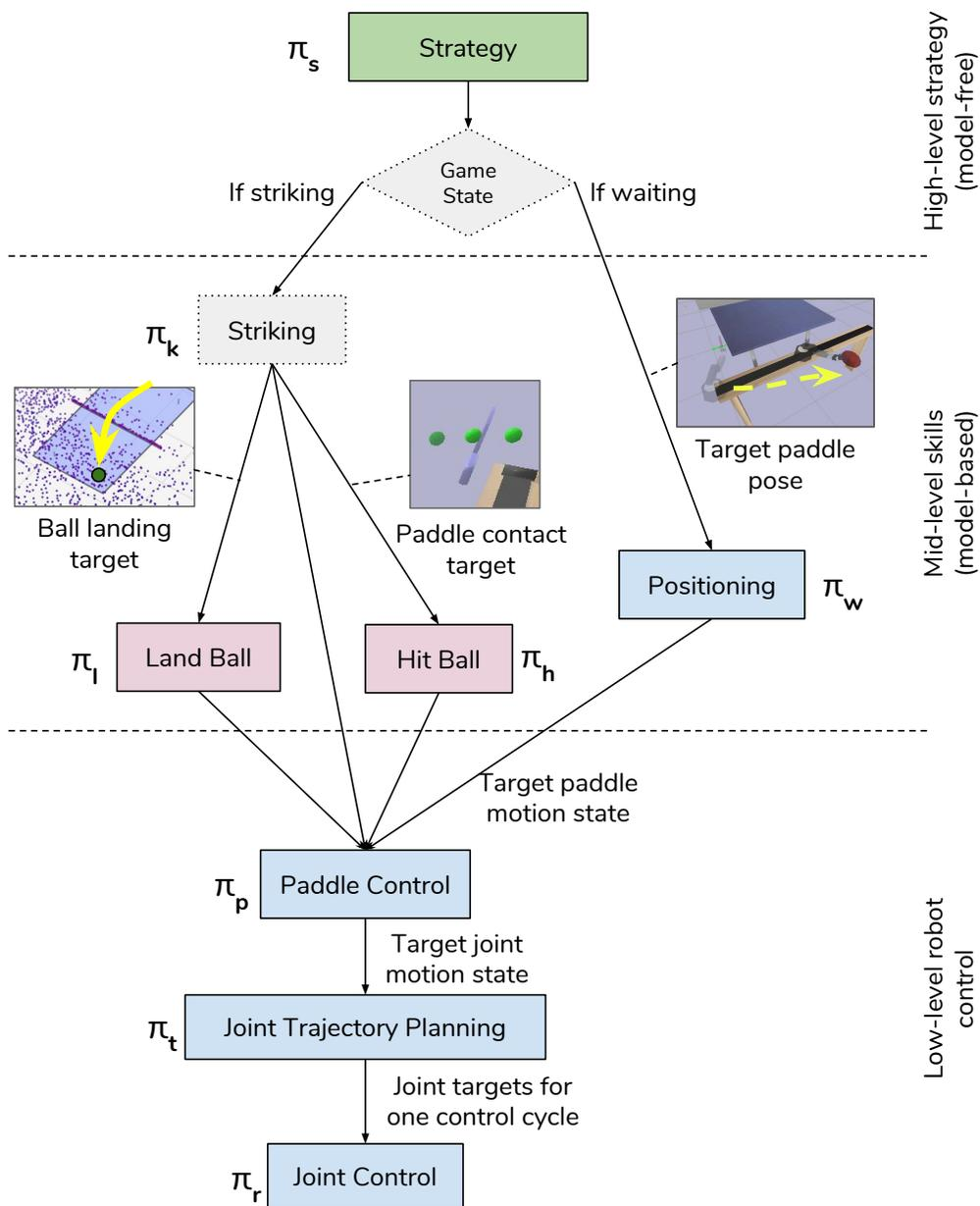
Figure 3.1: **The Skill Hierarchy.** The hierarchy consists of three levels of control (high-level, mid-level, and low-level), two modes (striking and waiting), and seven tasks. At any point in the game, the agent is either in striking mode or waiting mode. When in striking mode, the agent strikes the ball using one of three different skills: land-ball, hit-ball, or directly with paddle-control. Each variant of the policy uses only one of the three striking skills.
