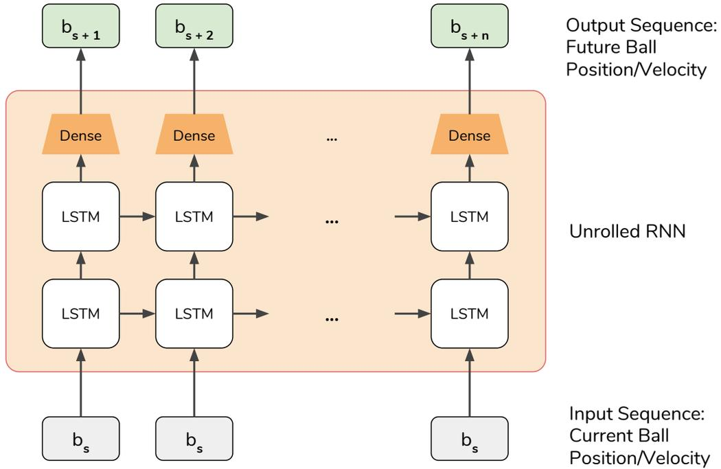
Figure 6.1: **Ball-Trajectory Prediction Model.** Given an estimate on the current position and velocity of the ball, predicts the future position and velocity of the ball over multiple timesteps. The recurrent model has two LSTM layers followed by a fully-connected layer. The figure shows the model unrolled through time for better visualization. At all timesteps, the model receives the same input  $b_s$ , which represents the current ball position and velocity.
