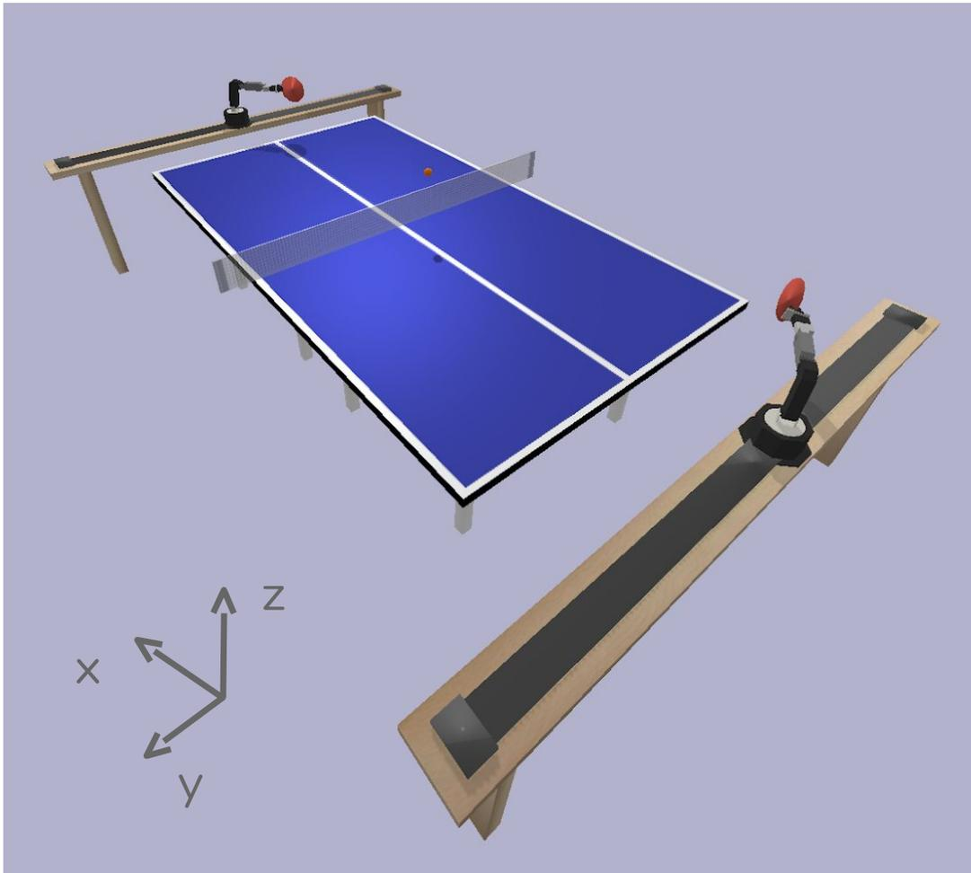
Figure 2.1: **Simulation Environment.** Two WidowX arms are mounted on linear actuators that allow the arms to move sideways. The two robot assemblies are at the same height as the table. The robot assembly consists of a linear actuator and a robot arm. The arm shown in the image is a WidowX arm with five joints. The original arm has a gripper, which has been removed in this setup and replaced with a fixed link holding a paddle.
