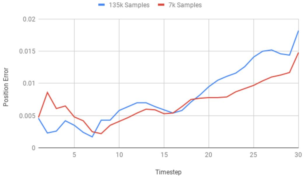
Figure 6.5: **Mean Position Error in Ball-Trajectory Predictions.** The plot shows the mean position error over 1000 ball trajectories containing 30 timesteps of observations each. The error reported is the Euclidean distance between the predicted position and the observed position of the ball. The average position error stays less than 1 cm after 25 timesteps, which suggests that the approach is effective.
