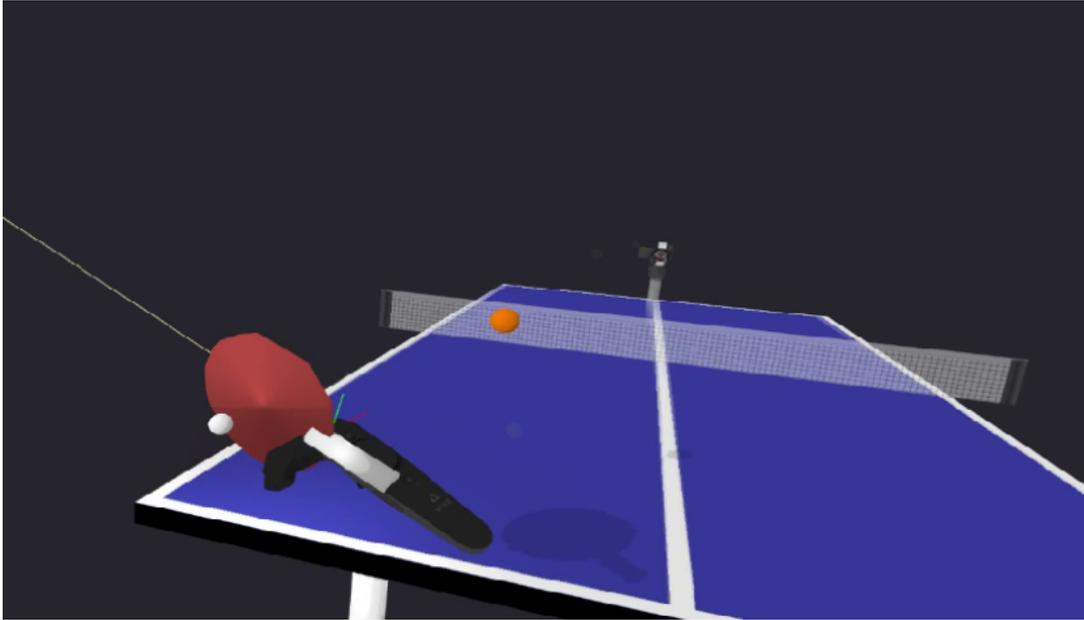
Figure 6.4: **Data Collection in VR Environment.** The VR environment allows a human player to control a simulated paddle by moving the VR controller in the real world. The simulated paddle follows the VR controller (visualized as the black object holding the paddle). The player returns the balls coming from a ball launcher on the other side of the table. The paddle and ball trajectories are recorded and used in training the dynamics models.
