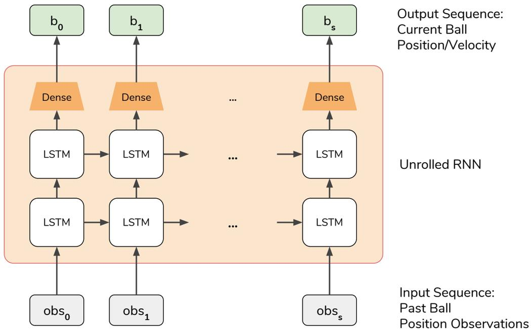
Figure 10.2: **Ball-State Estimation Model.** The current ball-motion state is estimated using a sequence model with LSTM layers followed by a fully-connected layer. The figure shows the model unrolled through time for better visualization. This model makes it possible to estimate the current position and velocity of the ball given a sequence of noisy position observations.
