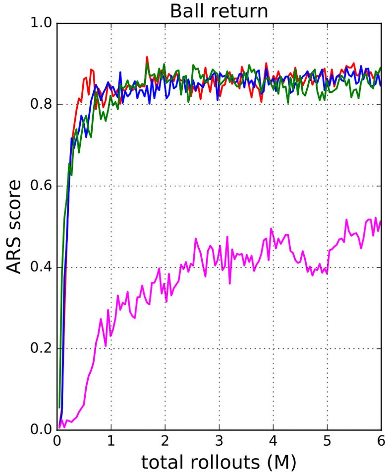
Figure 8.7: **Evaluation of Model-Free Return-Ball Policy Trained with ARS.** The four lines show the evaluation scores received from four different runs of ARS on the return-ball task. All runs use  $k = 15$ . Learning the policy with model-free RL requires  $\sim 1$ - $2$ M episodes. Such a high number of samples prevents using such algorithms on physical robots in the real world.
