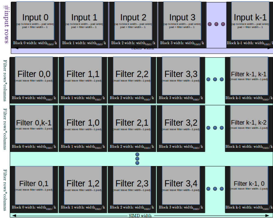
Figure 3.1: Basic ConvNet memory layout for both data and weight values. The first number in each green weight block is the filter group number, and the second number is the input channel number whose filter weights are stored in those SIMD rows. This layout arranges the data in a form to efficiently feed an implementation of the convolution algorithm that takes advantage of the hardware’s strengths, while minimizing its weaknesses.
